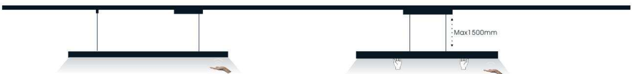
SDH-可选1/2 1.手扫切换上下光, 并调光 2.手扫切换色温, 并调光 SDH- optional 1/2 1.Hand sweep to choose direct light, indirect light or direct/indirect light, and hand stop for dimming 2.Hand sweep to change CCT in 3 steps (3000K/4000K/6000K), and hand stop for dimming
